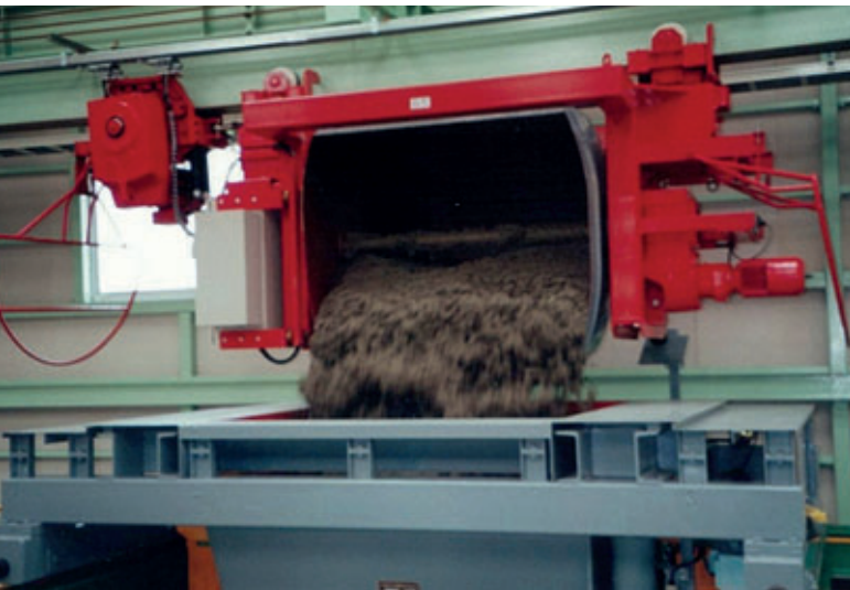
Fig. 6: TMD is feeding concrete to L-Crane Pouring Machine
